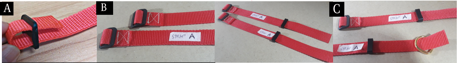
Attach the Slider to the strap. Fold the end strap and box stitch in place. Insert the Loop Keeper and D-ring on the other end of the strap
