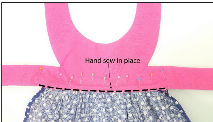
23. Pin Bodice Lining hem over waist seam and hand sew to cover seam.
